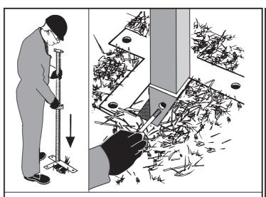
Compact or remove earth locally around the post to expose fixing bolt
